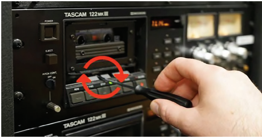
Figure 12. Making incremental turns to the left and right on a compact audio cassette player
