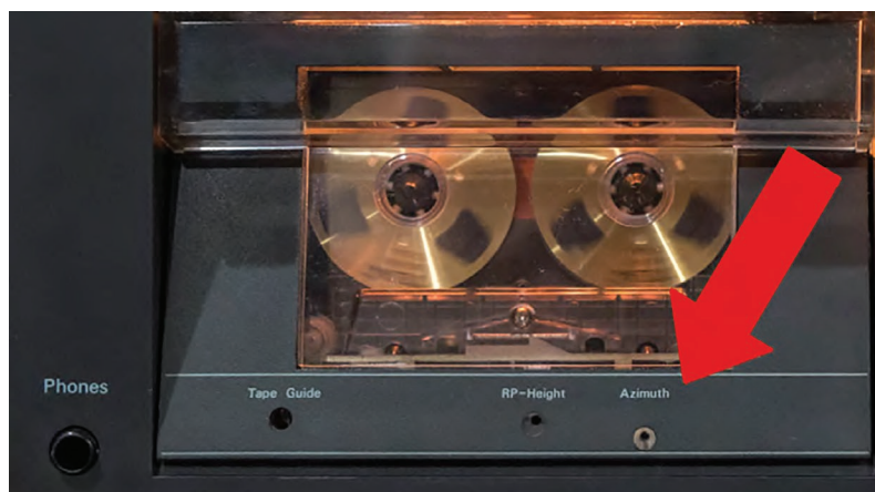
Figure 10. Example of Nakamichi 580 cassette deck with azimuth screw accessible from outside chassis
