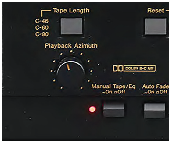
Figure 9. Dedicated playback azimuth control on Nakamichi CR-7E
