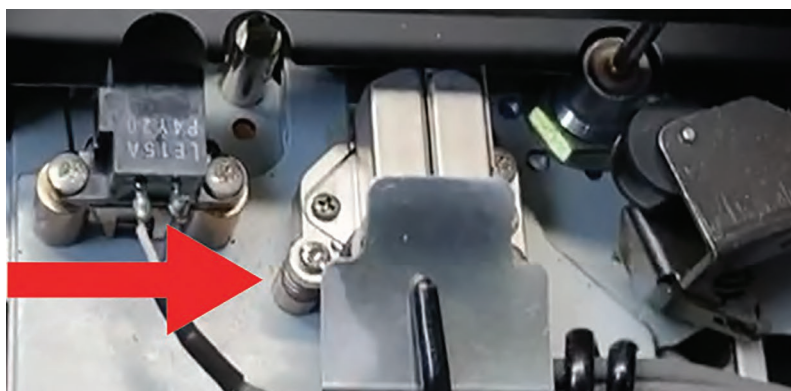
Figure 11. Closeup of azimuth screw in Tascam 122 MKIII with face plate removed
