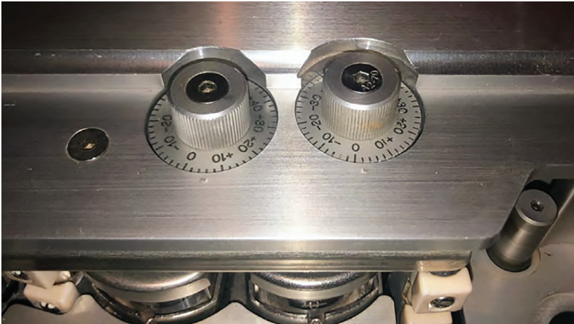
Figure 8. Azimuth dial controls installed on a Studer A80 open reel quarter-inch machine
